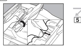
Open the Exit Guide while holding the green-labeled tab.
